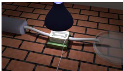
Figure 1. Reaction setup for the constant flow with a syringe-pump left-handed an outlet right-handed a UV-Lamp on the top, argon-inlet at the bottom of the picture and the reactor in the middle.
